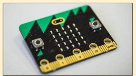
Small, programmable device. Includes an array of sensors, two buttons and 25 LEDs.
