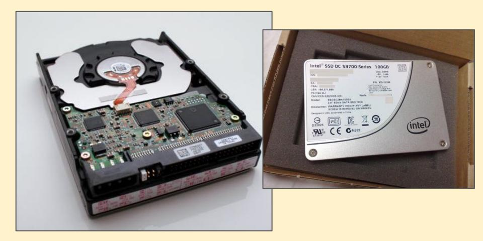
Hard Drives (left) and Solid State Drives (SSD) are used to store programs and data when the computer is turned off. Hard drives are bigger and cheaper. Solid State Drives are smaller but more expensive
