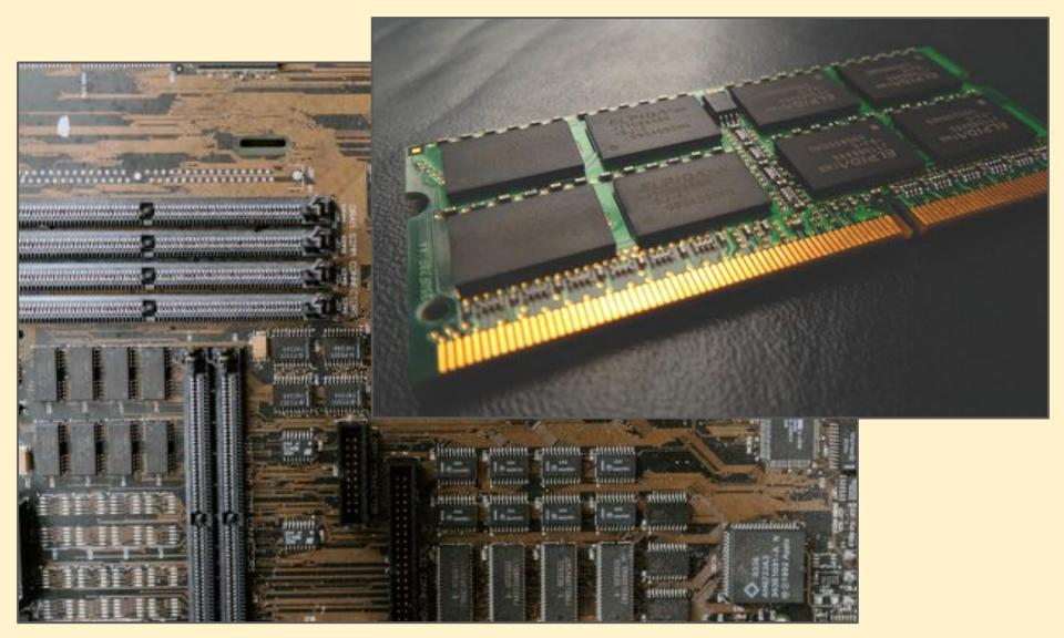
Random Access memory is te memory the computer uses to process. RAM cards slot in to the motherboard
