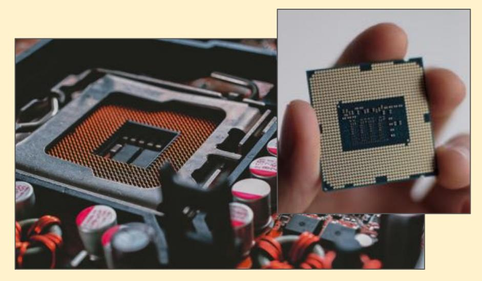
The **Central Processing Unit (CPU)** is the "chip" that makes everything work. This plugs in to the motherboard
