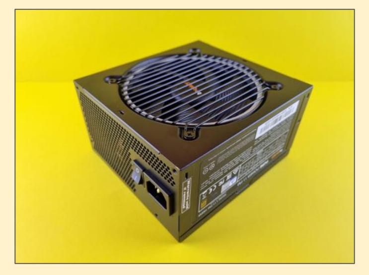
The Power Supply Unit provides electrical power to the computer at the right voltage. It usually includes a fan for cooling things down
